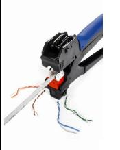
Zemecs T875A is a novelty product providing a comfortable and error free termination of Zemecs T481 (Category  $6_A$ ), T471 (Category 6) and T411 (Category 5e) series UTP 180° keystone jacks. It combines the advantage of punching 8 pins simultaneously by applying equal pressure and cutting excess wires at one go! Therefore contact stability is guaranteed and termination time is reduced up to 80%.
